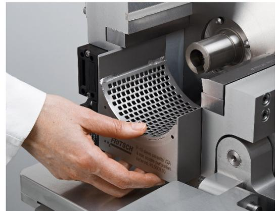
Fig. 1: Opened grinding chamber FRITSCH Cutting Mill
