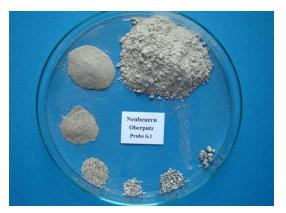
Fig. 3: Final plaster coat sample 6.1
