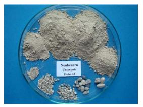
Fig. 5: Base plaster coat sample 6.2
