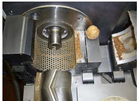
Fig. 3: The glance into the open grinding chamber shows an optimal throughput of the walnuts
