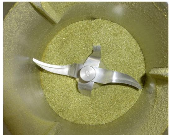
Fig. 2: Hops milled at 4,000 rpm, grinding time 15 seconds
