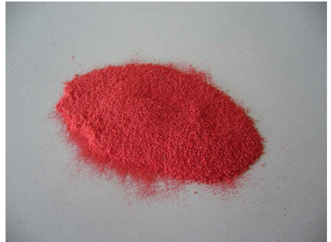
Fig. 4: Analytical fineness after milling with PULVERISETTE 14
