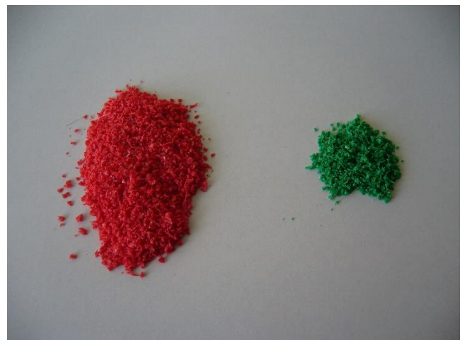
Fig. 3: Pre-grinding with PULVERISETTE 19, 2 mm sieve,
